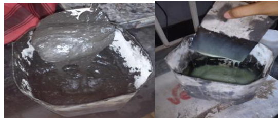
Figure2: Mixing of Measured Fly Ash, Resin and Hardener
