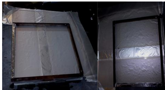
Figure 1: Wrapping of Aluminum foil to the Frame
