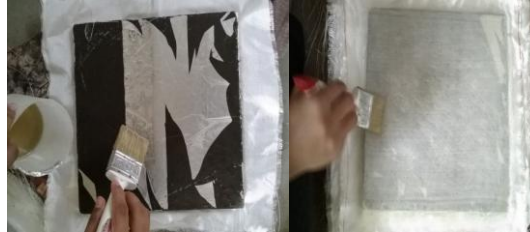
Figure 4: Bonding of Glass Fabric to the Core
